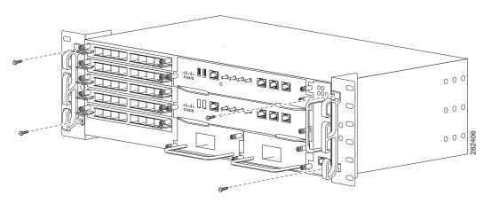
Step 2 Secure the cable management brackets with four M4 screws. The recommended maximum torque is 10 in.-lb (1.12 N-m).
